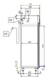
Electrical inlet (power) Refriaerant Inlet Refrigerant Outlet
